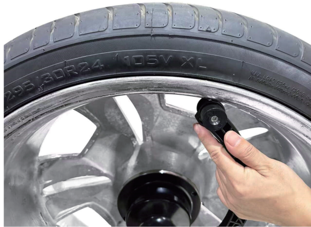
ALU-S balancing mode (balancing weight installation using the automatic measuring arm)
