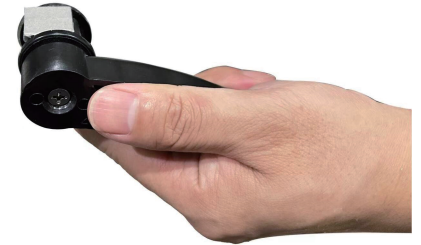
ALU-S balancing mode (balancing weight installation using the automatic measuring arm)
