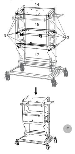
Find the below accessories with the serial number in the figure, lock NO.19 on the assembled F with screws, note the forward and backward placement of accessories, and finally form the figure G.
