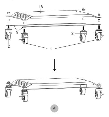
Find the below accessories with the serial number in the figure, and lock the screws as shown in the figure. Please pay attention to the placement of NO.4 screw and NO.3 screw during installation. NO.4 screw has a nut, please note the position of the nut, and finally form the figure B.
