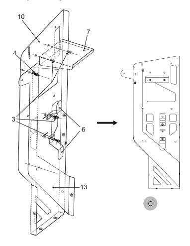
Install the assembled B and C on A as shown in the figure, and lock them with screws. Note the placement direction of B and C, and finally form the figure D.
