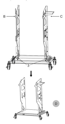
Find the below accessories with the serial number in the figure, lock NO.5, NO.8, NO.16 respectively on the installed D, note the forward and backward placement of accessories, and finally form the figure E.
