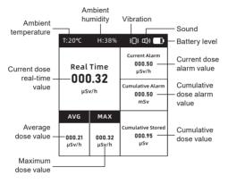
In the measurement interface, pressing the [ ◀ ] button or the [ ▶ ] button allows switching between measurement interfaces, as shown below:
