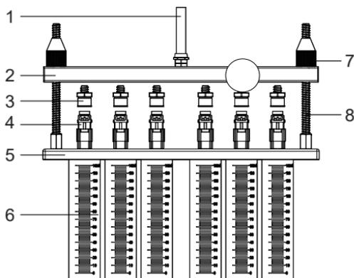
Top-in fuel injector installation diagram
